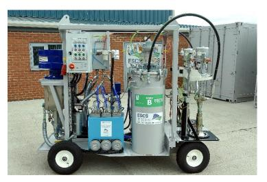
Cart Mounted Heated Airless Spray System. Suitable for the application All Major Solvent Free Plural Component Intumescent (PFP) Fireproofing Epoxies. The ES-430 is a compact unit built around supplying a complete proportioning system for the accurate mixing and application of PFP materials.
